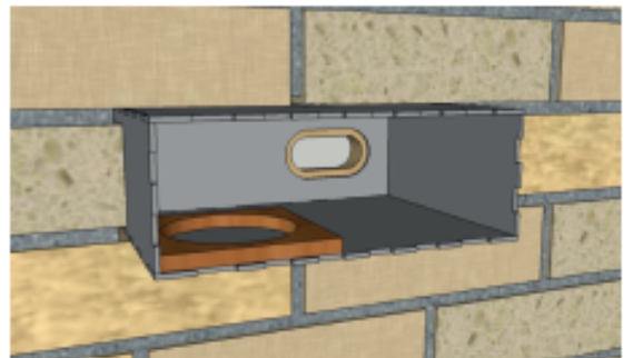
Cavity side with the back removed, showing the built-in nest form.
